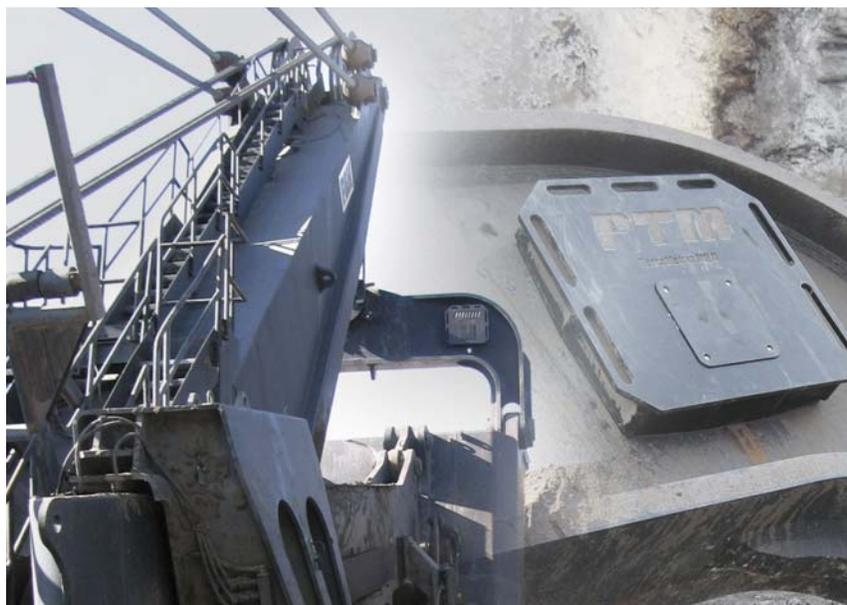
*A composite of a view of a rope shovel dipper and a close up showing the placement of the payload monitoring tool.*
